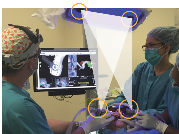
Figure 3 : Principle of the Dynamic Navigation System (Published with permission from Nobel Biocare). The spatial positions of the handpiece tracker (left yellow circle) and the patient tracker (right yellow circle) are determined via triangulation by two overhead cameras (upper yellow circles) tracking their respective positions.
