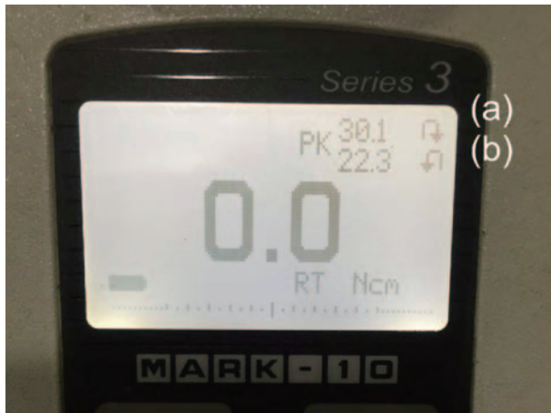
Fig. 3 Sample display of the torque-measuring machine (a) value of torque force (b) value of untorque force
