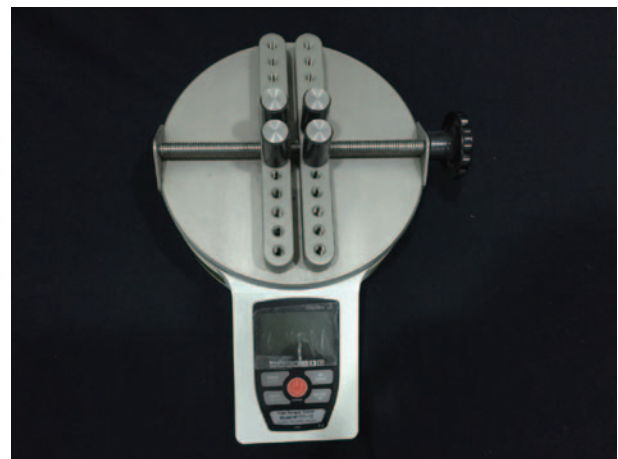
Fig. 2 Torque-measuring machine (Mark-10 model MTT01-12)
